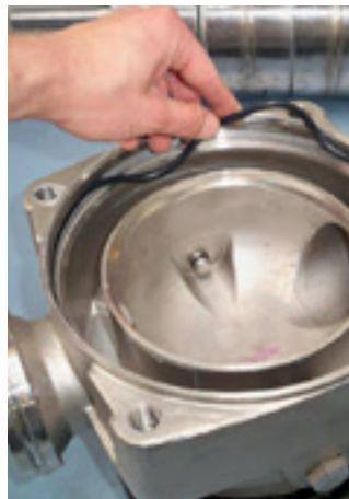
5. Coloque o anel o-ring na base com flange.
