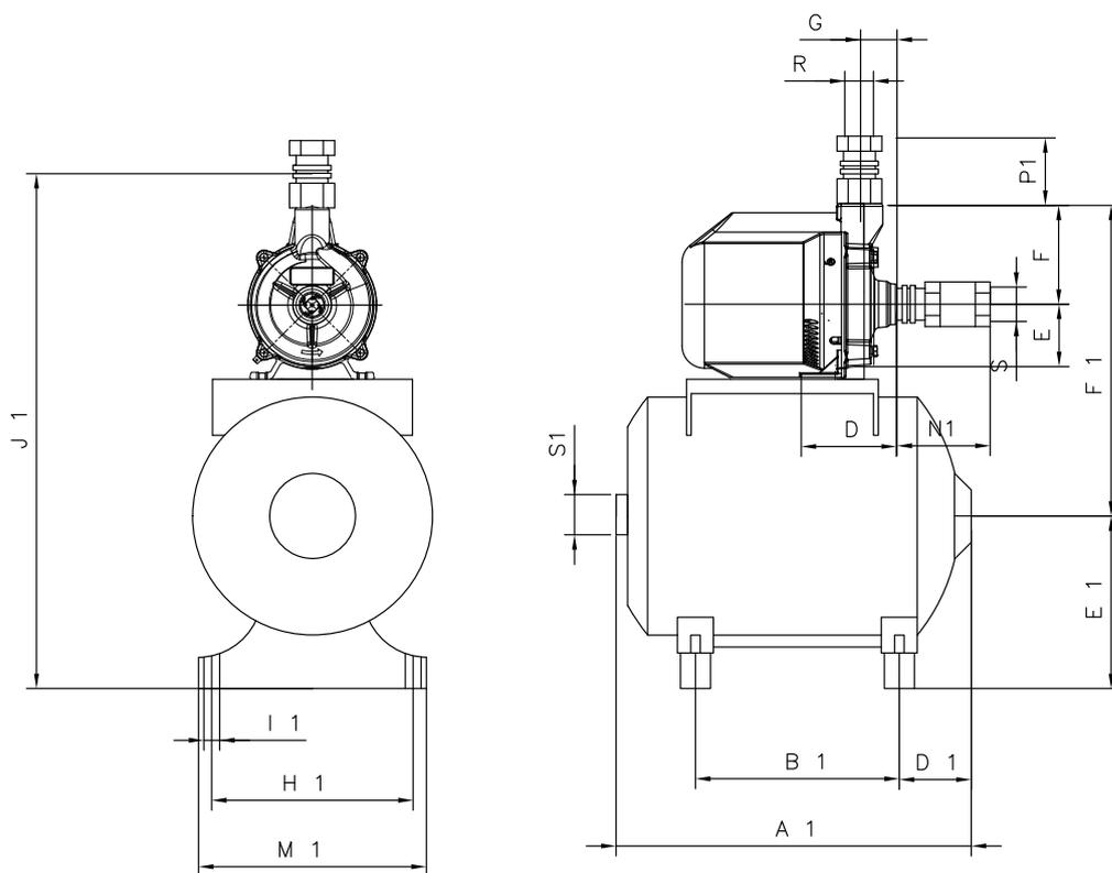
**DIMENSÕES EM MILÍMETROS (mm) - 60 Hz**
