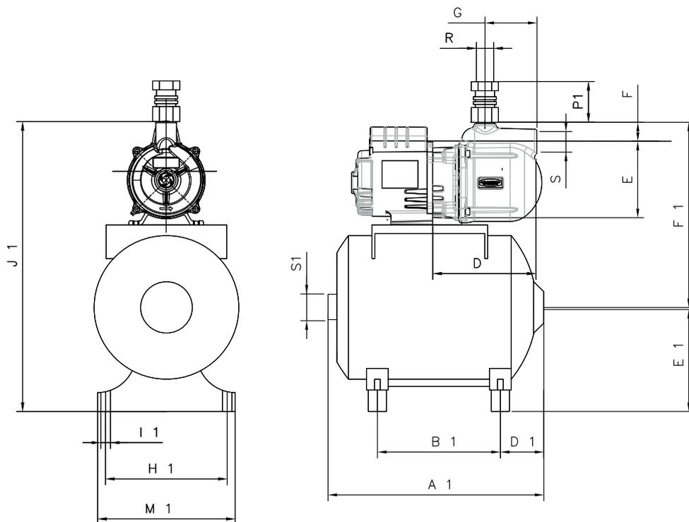
**DIMENSÕES EM MILÍMETROS (mm) - 60 Hz**
